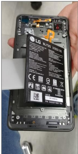
17. Lifts up the battery using the hera
