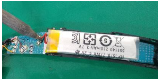
Remove battery wire.
