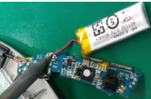
Remove battery wire.
