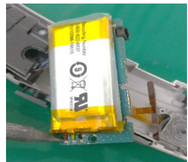
Remove battery wire.
