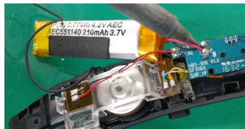
Remove battery wire.
