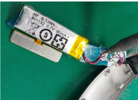
Remove battery wire.
