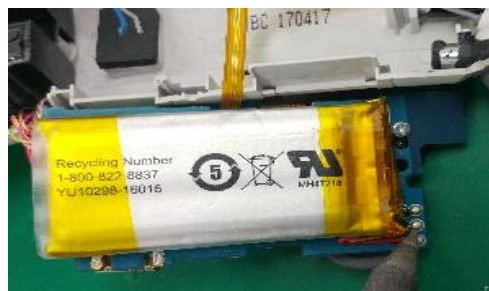
Remove battery wire.
