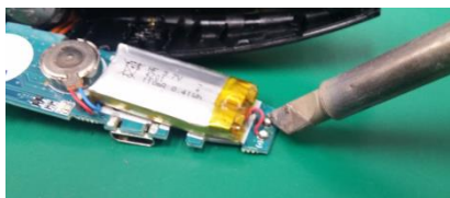
Remove battery wire.
