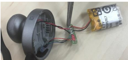
Remove battery wire.
