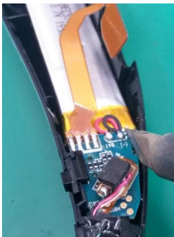
Remove battery wire.
