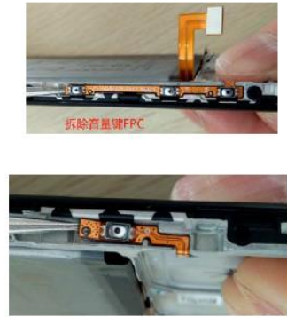
11.Side/Power key FPCB Remove
