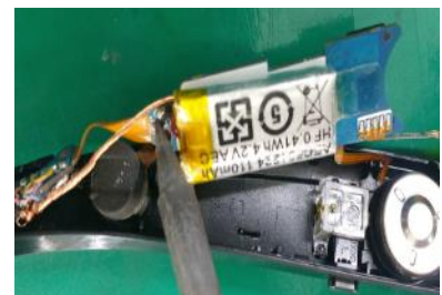
Remove battery wire.
